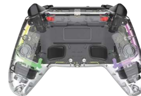
Adjustable Trigger with three levels of travel
