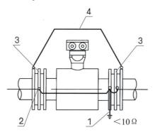
1. Ground device wire (install when external inference is stronger)
