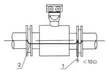
1. Ground device wire (install when external inference is stronger)
