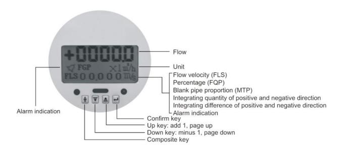
• Split III type keyboard definition and LCD display
