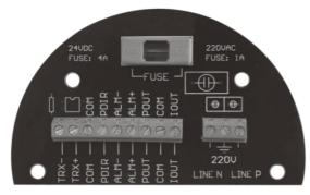
IOUT: Flow current output PUSE: Input power supply fuse COM: Current output place frequency (pulse) output place POUT: Bi-direction flow frequency (pulse) output TRX+: Communicating input
