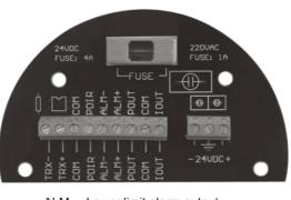
ALM-: Lower limit alarm output ALM+: Upper limit alarm output COM: Alarm output place TRX-: Communicating input
