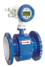
Installation modes: Flange integrated type Language selection: Chinese and English Aperture: DN10~DN800 Electrode material: 316, Hb, Hc, Ti, Ta Inside lining material: PTEE, PFA, F46, chloroprene rubber (CR) Medium: conducting liquid (include solid liquid two phase body) Accuracy grade: 0.2%, 0.5%, 1.0% (DN10~DN200) 0.5%, 1.0% (DN250~DN2000) Medium conductivity: > 5µS/cm (water > 20µs/cm)
