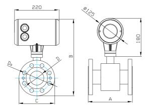
★ Note: Installation dimension for rubber liner the length need to increase  $6\sim10$ mm, for polytetrafluoroethylene liner the length need to increase 6mm; for split structure; on the converter position in the diagram want to install wiring box, i.e. take wiring box replace the converter and take converter single separately mount on the wall or support frame.
