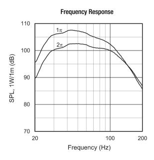
1 watt at 1 meter, with 150 Hz Linkwitz-Riley 4th order low-pass filter and 2nd order high-pass filter at 25 Hz with Q=2. 1pi (upper curve) and 2pi (lower curve) conditions.
