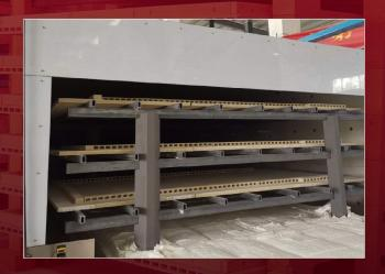
The setter batts used in roller kilns for the firing of ctystallized glass panels should have both a large surface area and at the same time a thin cross section. The firing cycle in a roller kiln is generally faster than in a tunnel or shuttle kiln. Therefore the thermal shock resistance of batts is very important.
