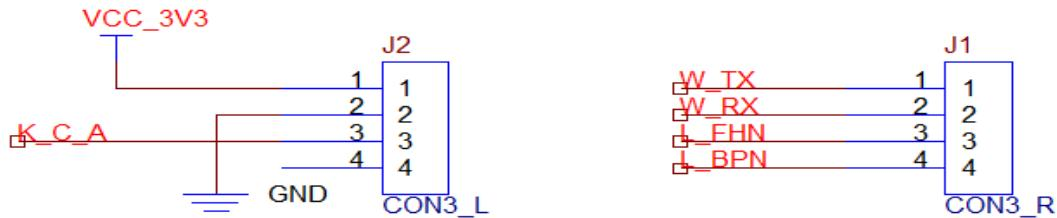
If the screen printing are the same, W\_TX , W\_RX connect the serial port of the module, L\_FHN , L\_BPN connect the IO of the module respectively.
