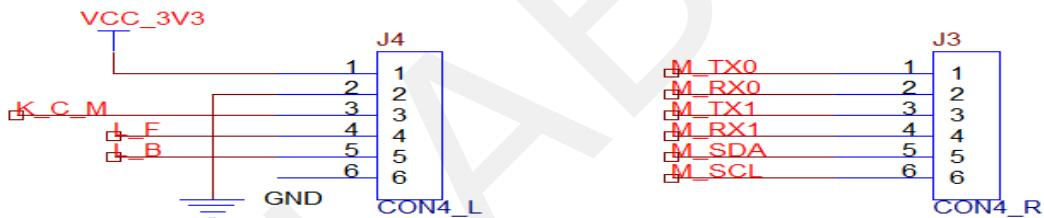
If the screen printing are the same, M\_TX0 , M\_RX0 is MCU serial port 1 , M\_TX1, M\_RX1 is MCU serial port 2 , M\_SDA , M\_SCL is Optical drive interface (IIC)
