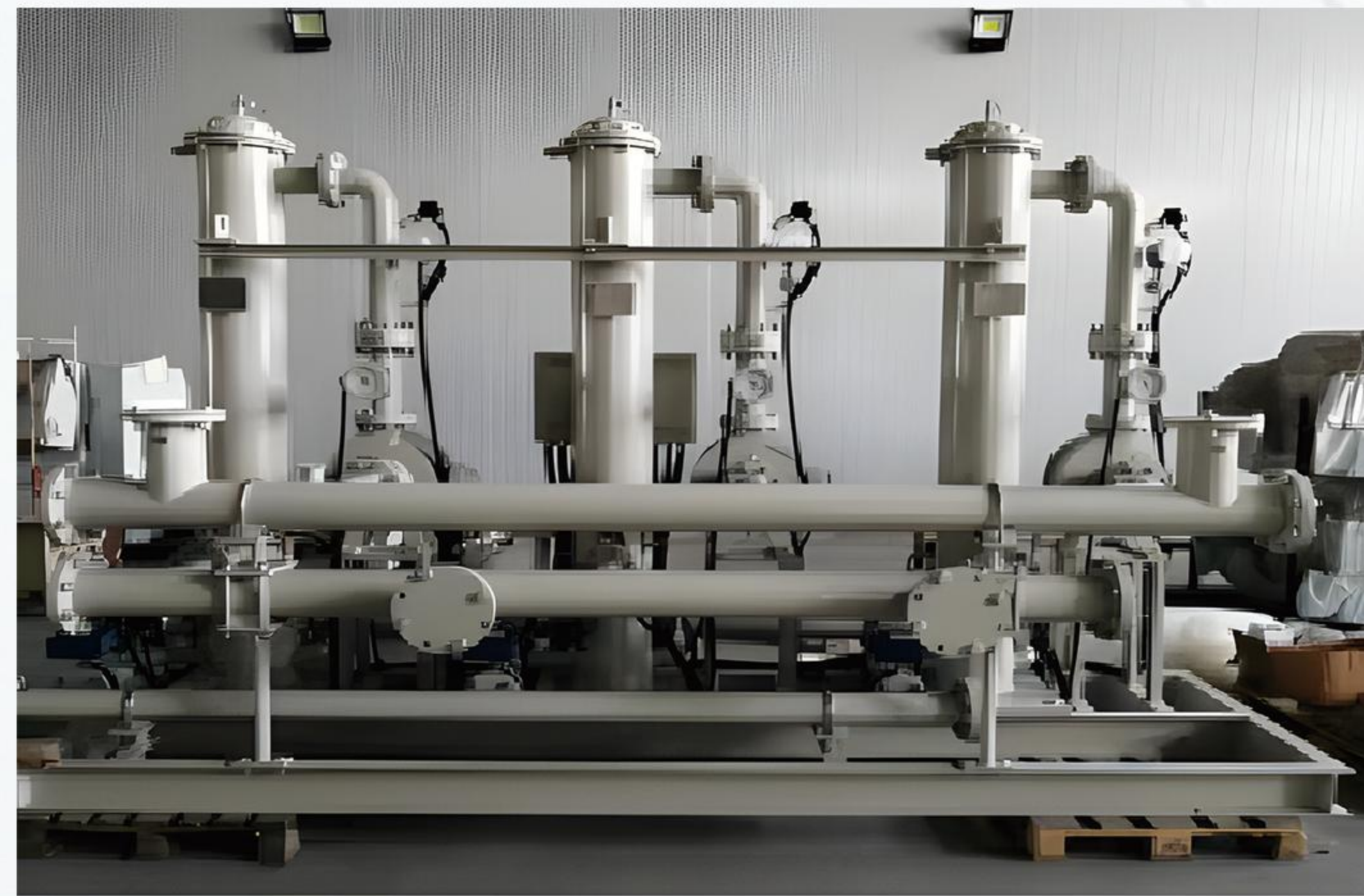
油水冷却器应用于巴基斯坦苏基纳里水电站单机容量为 221MW 的冲击式水轮发电机组 OFWF applied to pakistan sukkiknari hydropower station, whose impulse turbine generator unit has the unit capacity of 221MW
