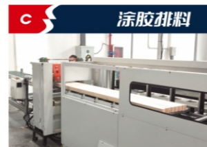
After fine planing, the wood enters the gluing and automatically discharges
