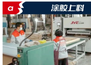
The glue applicator applies glue to two panels
