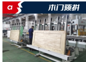
Wooden door parts pre-assembled Automatic flip to the assembly line
