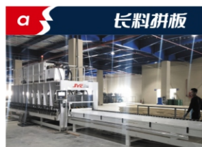
a 长料拼板 Suitable for long material joining Realize segmented continuous joining
