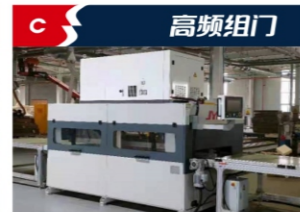
Wooden doors are assembled by HF heating, Fast-curing glue
