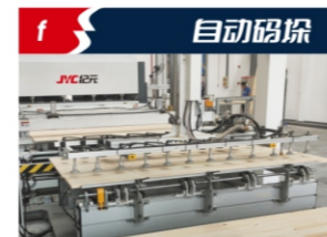
Gantry suction cups will palletize the sawn boards.
