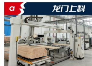
Floor rollers send the wood to the Gantry feeding machine for feeding
