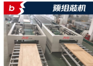
Assembled wooden door is pressurized and normalized to ensure tightness
