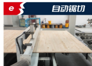
The board is flush with the edge, and the transverse sawing is precise
