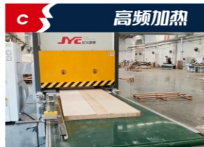
Fast curing of glue for upper and lower panels of wooden doors
