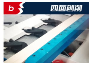
The wood is planed on all sides. Bottom /inside/outside/upper fine planing
