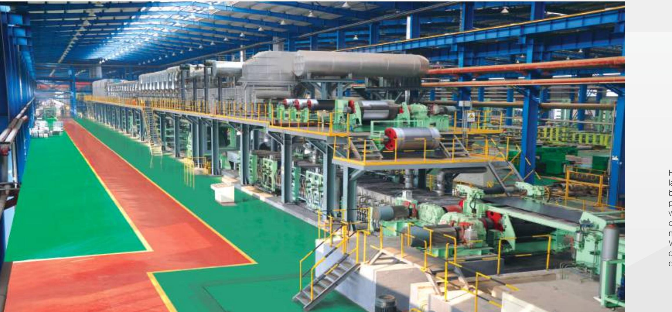
Hot galvanizing/ galvalume is coating one layer of zinc or sibley alloy on strip surface by hot dipping which has strong cathodic protection performance and has been widely used in manufacturing, agriculture, construction and others. It has become the most useful plating product nowadays. We have built up over two hundred hot dipped galvanizing/ galvalume lines in domestic and overseas.
