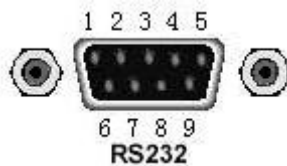
Figure 5-1 Rear Panel RS232 Interface
