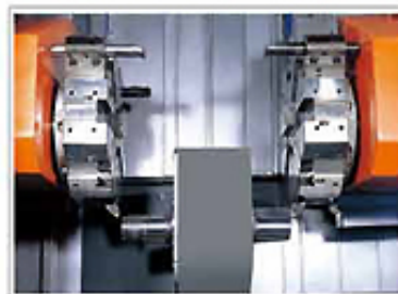
短工件可以單主軸夾持 Short workpiece clamped by single spindle.
