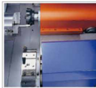
車削後CNC切角成型 CNC polygon cutting after turning.
