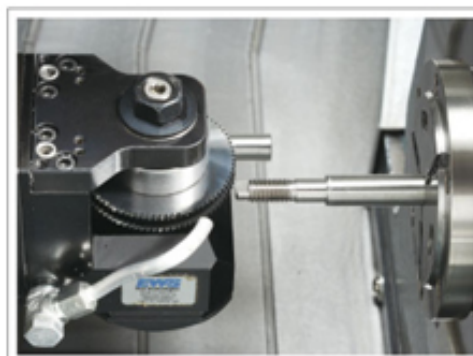
▲ 動力刀塔銑2、4、6平面(選備) Power turret with radial saw flat milling by 2,4,6 sides. (Option)
