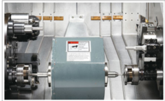
▲ 機上兩端各別滾牙(選備) Both ends threading function (Option).
