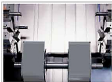
兩台主軸夾持長度800mm Max. Clamping length of twin spindle is 800mm.
