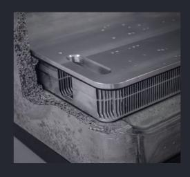
The projector's core is the floating heatsink mounted on a flexible seal in the chassis. This construction helps to reduce vibrations and allows the heatsink to overcome heat expansion without the risk of deformation.
