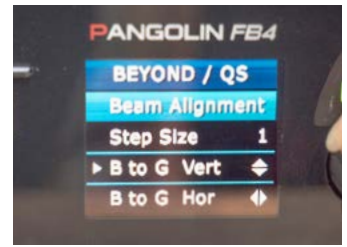
D: Here you can set the STEP SIZE ( amount of movement in a single step ), and VERTICAL / HORIZONTAL movement for every colour in your projector ( R=RED, G=GREEN, B=BLUE, Y=YELLOW ).
