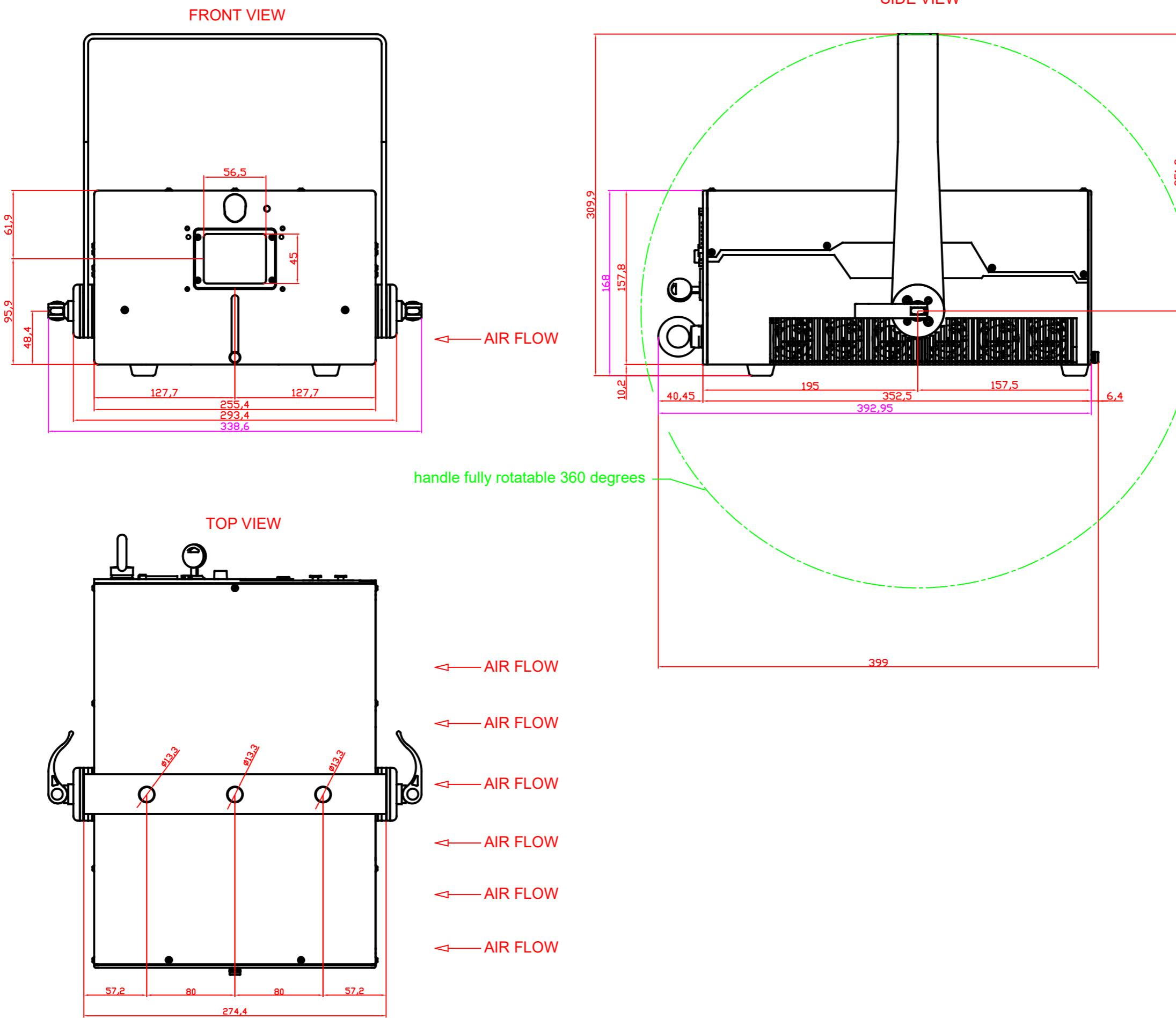
Purple: Overall dimensions, including all the fittings and extrusions; without the 360° swivel bracket
