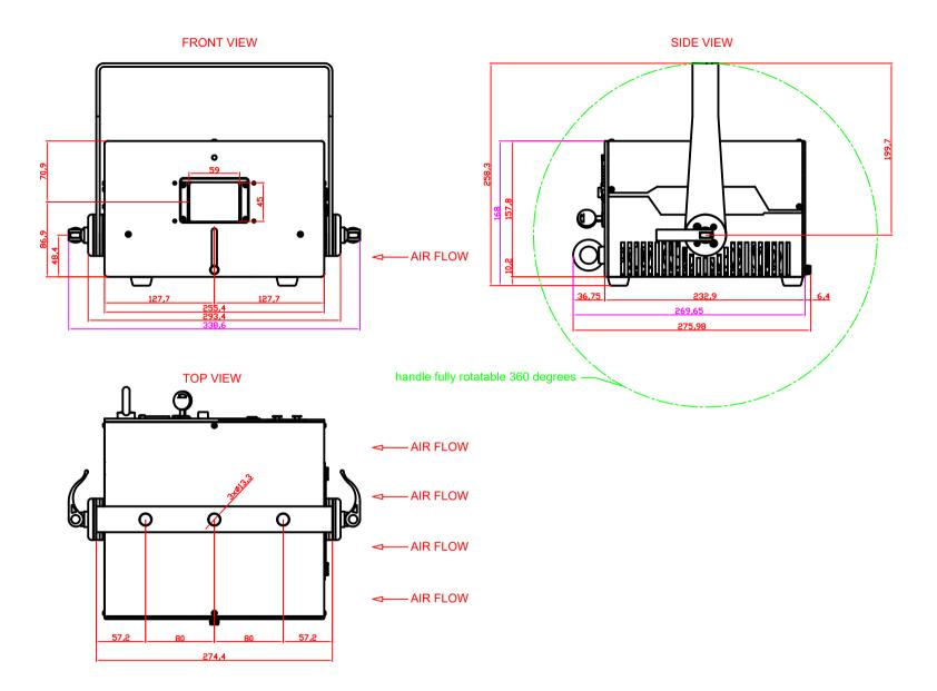
Purple dimensions means general dimension of laser projector Tottaly air flow for laser projector: 40 squere meter per hour
