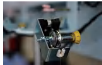
单纱多级张力器 Multistage single yarn tensioner
