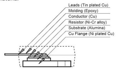
Between flange and resistor are insulated
