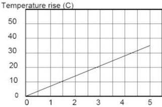
Applied Power (W) Rating Power(W), with 2.8K/W heat sink.
