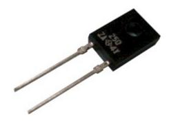
These are TO126 super precision power resistors. They can achieve 1W in free air and 5W when attached to the copper foil of a circuit board. These models exhibit low noise, high frequency operation and high density installation. Applications include: Constant current sources, electronic load circuits, LSI tests, measurement, audio PA systems and motor control.
