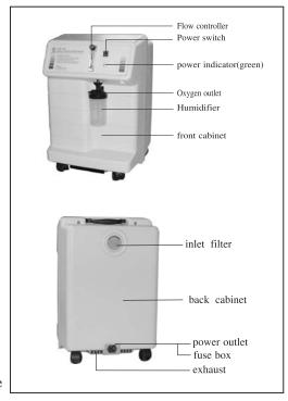
oxygen concentrator. The oxygen will be moistened by the humidifier, it will flow out of outlet of the upper-cover. Nasal cannula should attach to the humidifier outlet port. There is a safety valve on the humidifier cover, whose pressure is  $0.02\pm0.005$ MPa.
