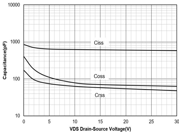
Figure 3. Capacitance Characteristics
