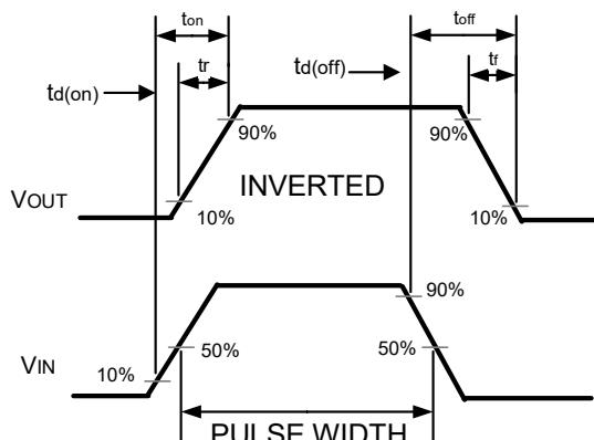
Figure 10. Switching wave
