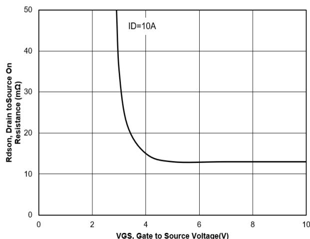
Figure 7. Typical Drain to Source ON Resistance
