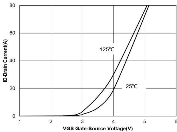
Figure 2. Transfer Characteristics
