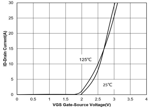
Figure 2. Transfer Characteristics
