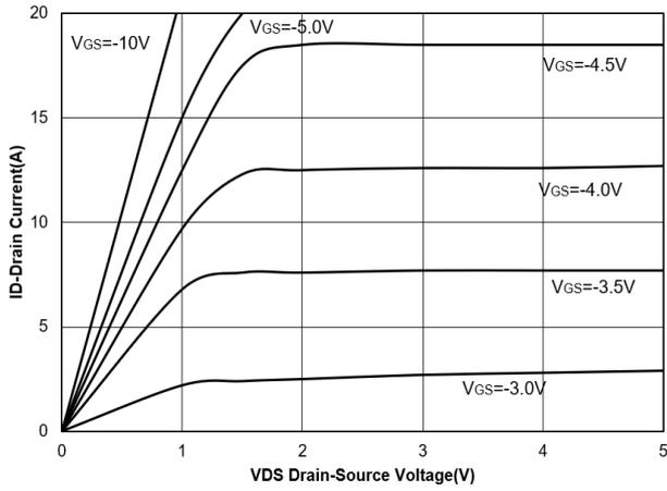
Figure 1. Output Characteristics
