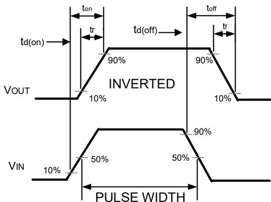
Figure 10. Switching wave
