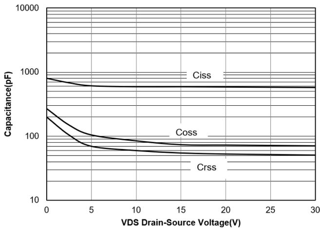
Figure 3. Capacitance Characteristics
