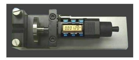
The KD-CH-IIID is a precision fixture that secures a non-contact displacement sensor and accurately varies the position of a target relative to the sensor. It provides and excellent means of obtaining calibration data at the user' facility
