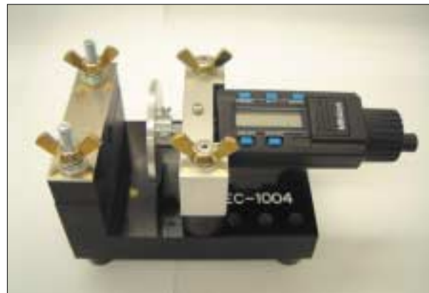
AEC-1004 Calibration range: 0 to 25 mm Minimum scale indication: 1 \mu m (digitally displayed)
