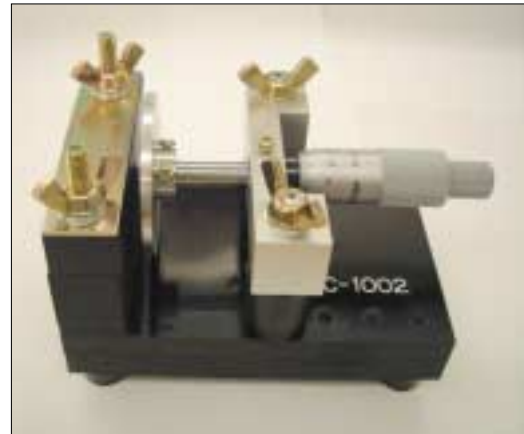
AEC-1002 Calibration range: 0 to 25 mm Minimum scale indication: 10 \mu m
