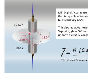
MTI Digital Accumeasure amplifier is a multichannel digital capacitance gauge that is capable of measuring thickness of semi-insulating wafers such as high
