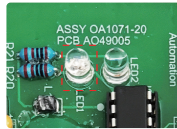
电路板故障指示灯
