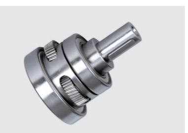
出轴表面磨削处理，与油封搭配确保低摩擦，从而减少了启动负载，保持最佳的密封性，延长了使用寿命。Grinding process to smooth surface of output shaft, and with oil-seal to minimum friction coefficient and reducing start up load; result in the best seal-ability and extended lifespan.
