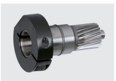
输入端与电动机转轴的连接采用栓紧式机构，锁紧环经过动平衡分析，确保在高转速下两结合面的同心度和相对零转动。Input-end and motor shaft are coupled through a dynamic balanced collar clamping mechanism to ensure connection interface concentricity and zero slip power transmission at high speed.
