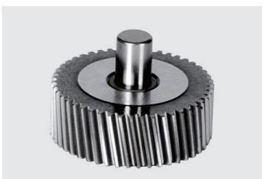
行星齿轮传动采用滚针轴承，满针排列不含保持架，以达到最大接触面积和最小间隙，提高了结构刚性和输出扭力。Planet gear transmission interface equipped with needle bearings, full needle roller bearings aligned without retainer achieve maximum exposure but smallest gap tolerances. Enhance over-all gear structure rigid and output torque.
