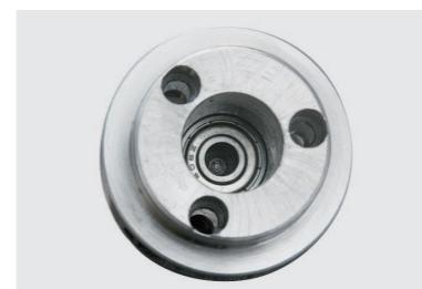
太阳齿前端轴承直接置于行星固定架内，整体机械结构设计，以确保传动元件的同心度。The sun gear bearing is placed directly into the planetary arm bracket, the overall mechanical structure designed to ensure concentricity of the transmission components.
