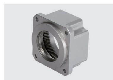
齿轮箱与内环齿一体设计，经插齿机加工齿部。具有高精度，高扭力，高耐磨等特点。The gear box and internal gear ring are one-piece part, and processed with gear shaper machinery for high precision, high torque and abrade consumption.
