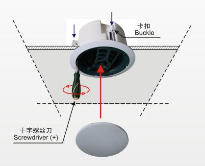
3) 将音箱装入安装孔内,用螺丝刀把四个卡扣锁紧,再将喇叭网装上即可。 Install the speaker into the hole and fix the four buckles with a screwdriver, and then install the netting.
