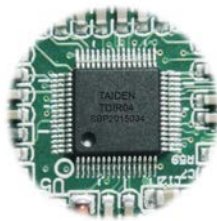
TAIDEN TDIR04 digital infrared processing chip
