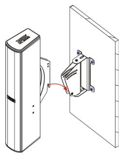
5. Set the tilt angle: if the speaker has nested securely on the pivot bolt, disassemble the PM6×35 mm bolt in the top of the bracket, and then slide it into one of the holes in the top of the wall bracket.
