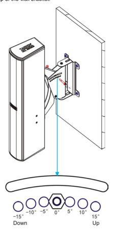
6. Set the swivel (pan) angle: loosen the top and bottom bolts on the pivot, adjust swivel aiming angle of the speaker, then tighten the bolts
