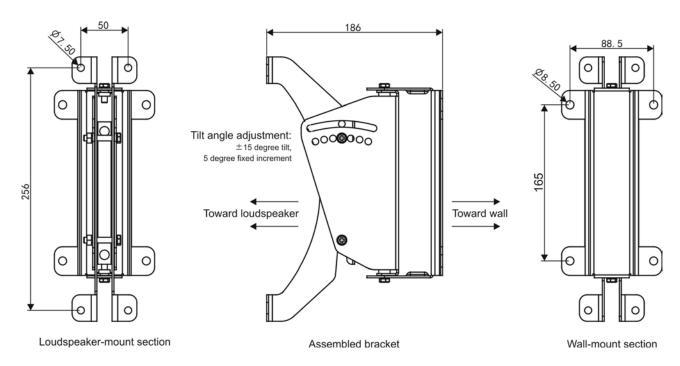
Dimensions of swivel (pan) / tilt wall bracket (unit: mm)
