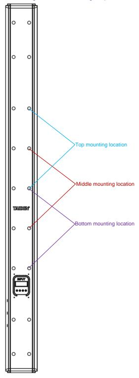
HCL-1800U (top half) and HCL-1800D(bottom half) Line Array Column Loudspeaker needs to be firmly connected by coupler plate, and then fixed the speaker bracket onto the coupler plate (ONLY fixed on coupler plate, not on other mounting location), and it supports ±80 degree swivel (pan) and ±5 degree tilt angles
