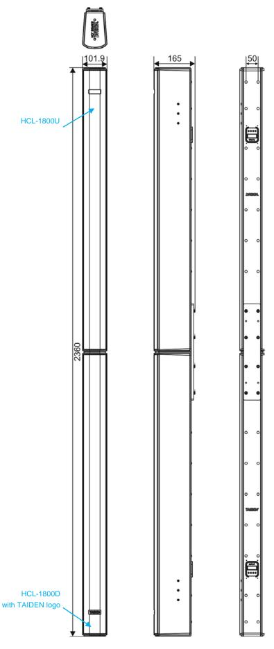
Dimensions of HCS-1800U+HCL-1800D Line Array Column Loudspeaker (unit: mm)
