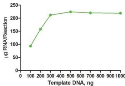
Fig 3. Relationship between the input and yield of 1.4 kb template
