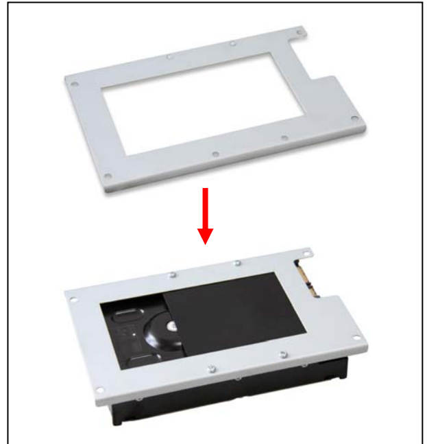
Figure 1.4 Installation of the bracket onto the harddisk
