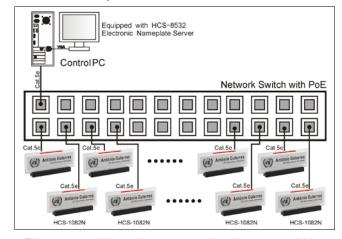
Figure 2.3.3 Nameplates connection via cat.5e cable (without main unit)
