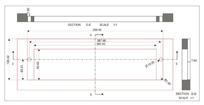
Figure 2.2.3 Fixing hole positioning diagram of HCS-1082S(N)/FM (unit: mm)
