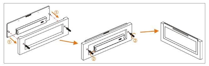
Figure 2.2.4 Flush-mounted installation of the HCS-1082S(N)/FM
