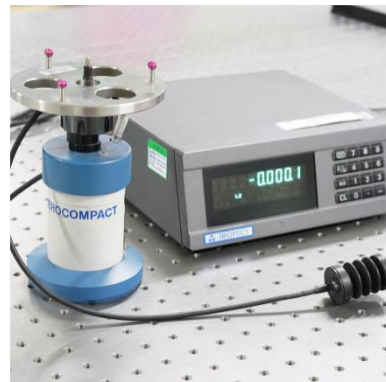
Trioptics Spherometer for radius of curvature measurement
