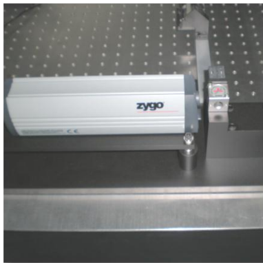
ZYGO Interferometric Radius Slide System(IRS, based on ZMI): measure radius of curvature with high accuracy Resolution: 10nm Accuracy: greater than 3\mu\text{m} or 0.001%
