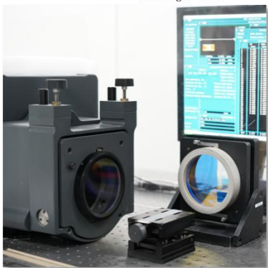
ZYGO Interferometer for wave front & parallelism Measurement With \lambda/50 accuracy Parallelism measure accuracy: 0.5''
