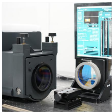
ZYGO Interferometer for high accuracy measurement of wave front & flatness & parallelism With \lambda/50 accuracy Parallelism measure accuracy: 0.5''
