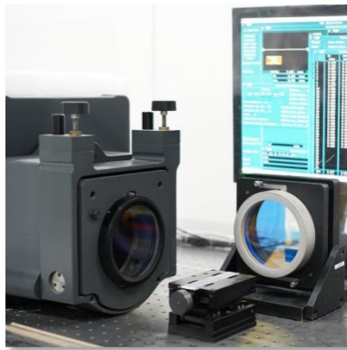
ZYGO GPI-XP Interferometer for wave front & parallelism measurement With \lambda/50 accuracy Parallelism measure accuracy: 0.5 "
