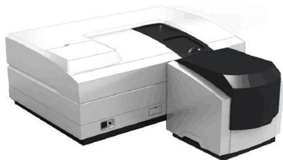
Agilent Cary-7000 (2sets) for reflectivity testing from 175nm to 3300nm spectral region
