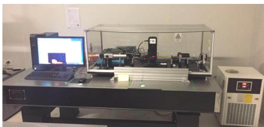
1064nm laser damage threshold testing system(CW,100W)
