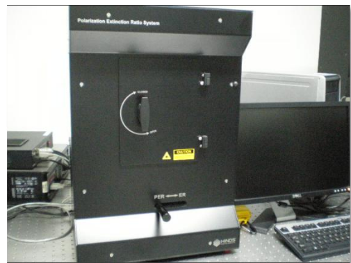
Extinction Ratio Measurement PER:>50dB ER:>250000:1
