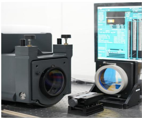
ZYGO Interferometer for wave front & parallelism measurement with \lambda/50 accuracy Parallelism measure accuracy: 0.5 "
