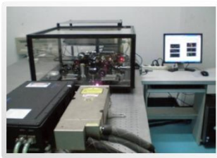
Surface absorption testing by PCI (355nm,532nm,1064nm)
