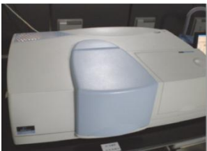
Perkin Elmer Lambda-950 for 175-3300nm spectral region
