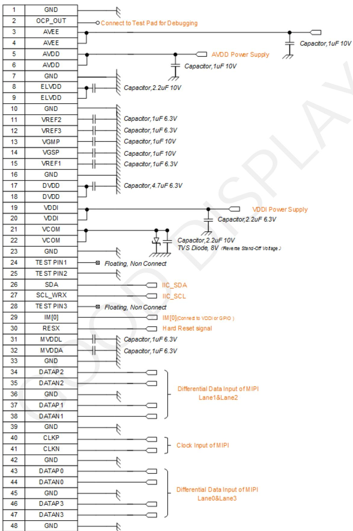
Mounting the capacitor for each power supply to ensure that the panel display normally.
