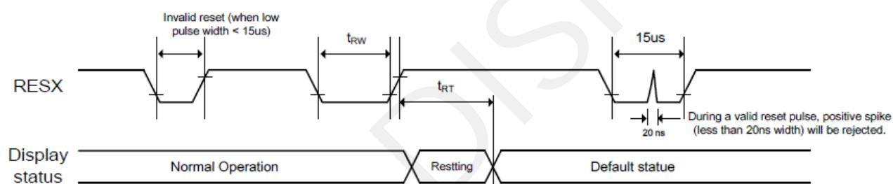
Reset time @ VDDI=1.65V to 1.95V, AVSS=VSS=MVSS=0V, Ta=-40°C to 85°C
