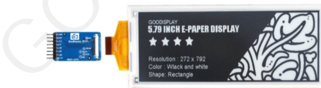
Figure 4.1 Connection between DESPI-C579 and e-paper display
