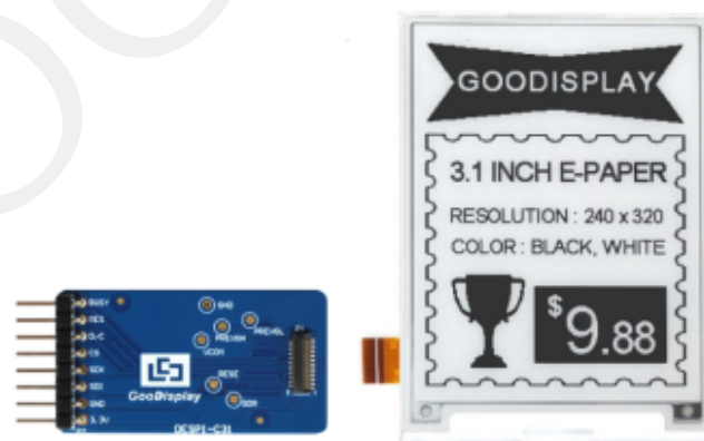
Figure 4 Connection between DESPI-C31 and e-paper display
