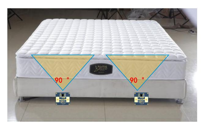
The radar can also be placed under the mattress, for double beds, we recommend installing two radar modules to measure the sleep status of each person
