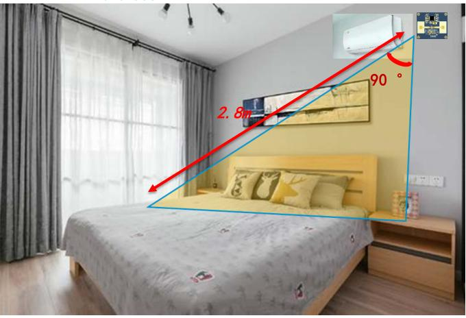
When the sleep radar is measuring human activities, there should be no obstruction between it and the human body. The effective distance of measuring is 2.5 meters, and the antenna emits in a 90-degree circle. The radar output signal is: somebody, awake, light sleep, deep sleep, nobody, apnea alarm information
