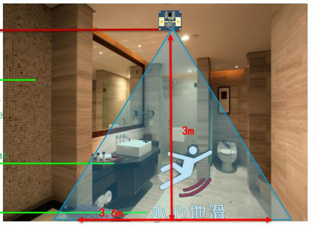
The fall radar needs to be installed above the bathroom. The antenna of the radar is facing down. If the toilet is 2 meters high, the measured diameter is 2 meters. If the toilet is 3 meters high, the measured diameter is 3.6 meters.
