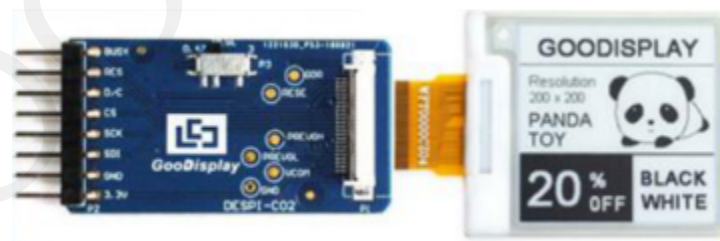
Figure 4 Schematic diagram of e-paper and adapter board plugging
