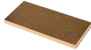
<All surface covered with copper>
