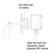
Use suitable cable glands or conduit system. Not used entries have to be closed tight.
