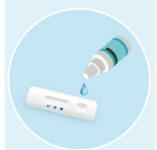
Add 2-3 drops of buffer solution to sample port
