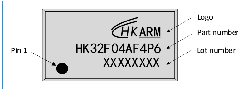
Figure 6-22 TSSOP20 HK32F04AF4P6 marking example
