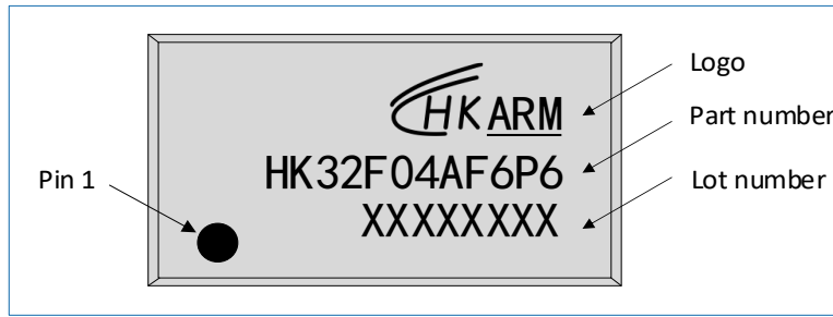
Figure 6-21 TSSOP20 HK32F04AF6P6 marking example
