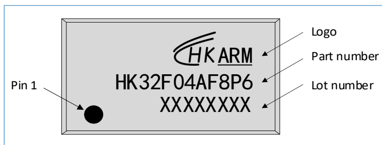
Figure 6-20 TSSOP20 HK32F04AF8P6 marking example
