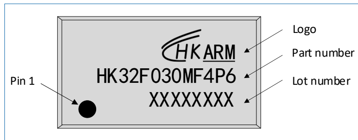
Figure 7-10 TSSOP20 HK32F030MF4P6 marking example
