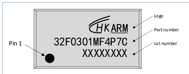
Figure 7-8 TSSOP20 HK32F0301MF4P7C marking example
