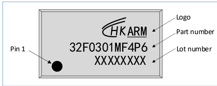
Figure 7-10 TSSOP20 HK32F0301MF4P6 marking example
